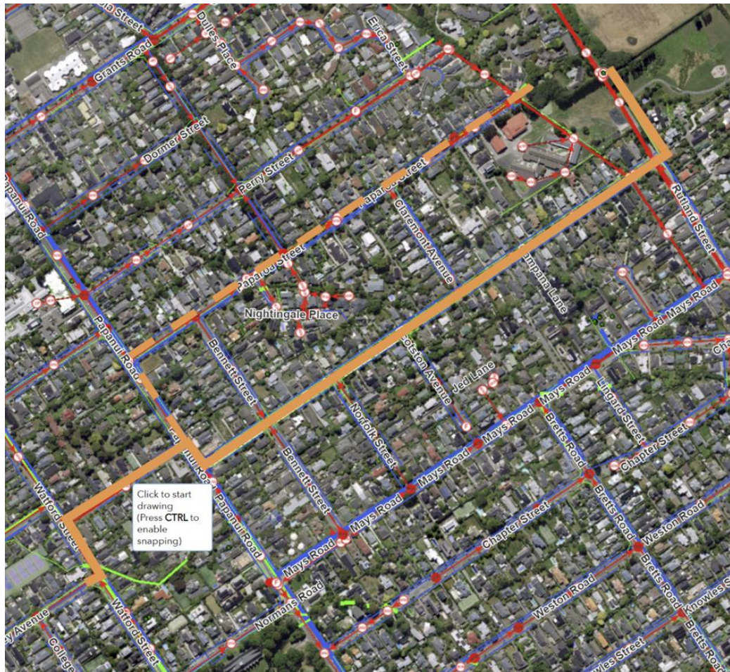
Figure 2: Indicative pressure main alignment
