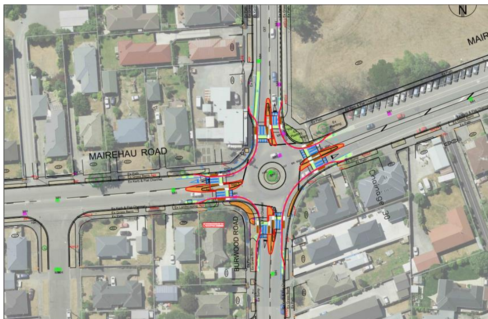
Figure 5: SIDRA Model – Upgraded Roundabout Layout
