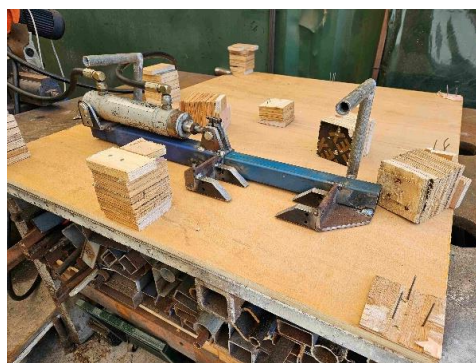
Hydraulic ram designed & built for dismantling pallets
