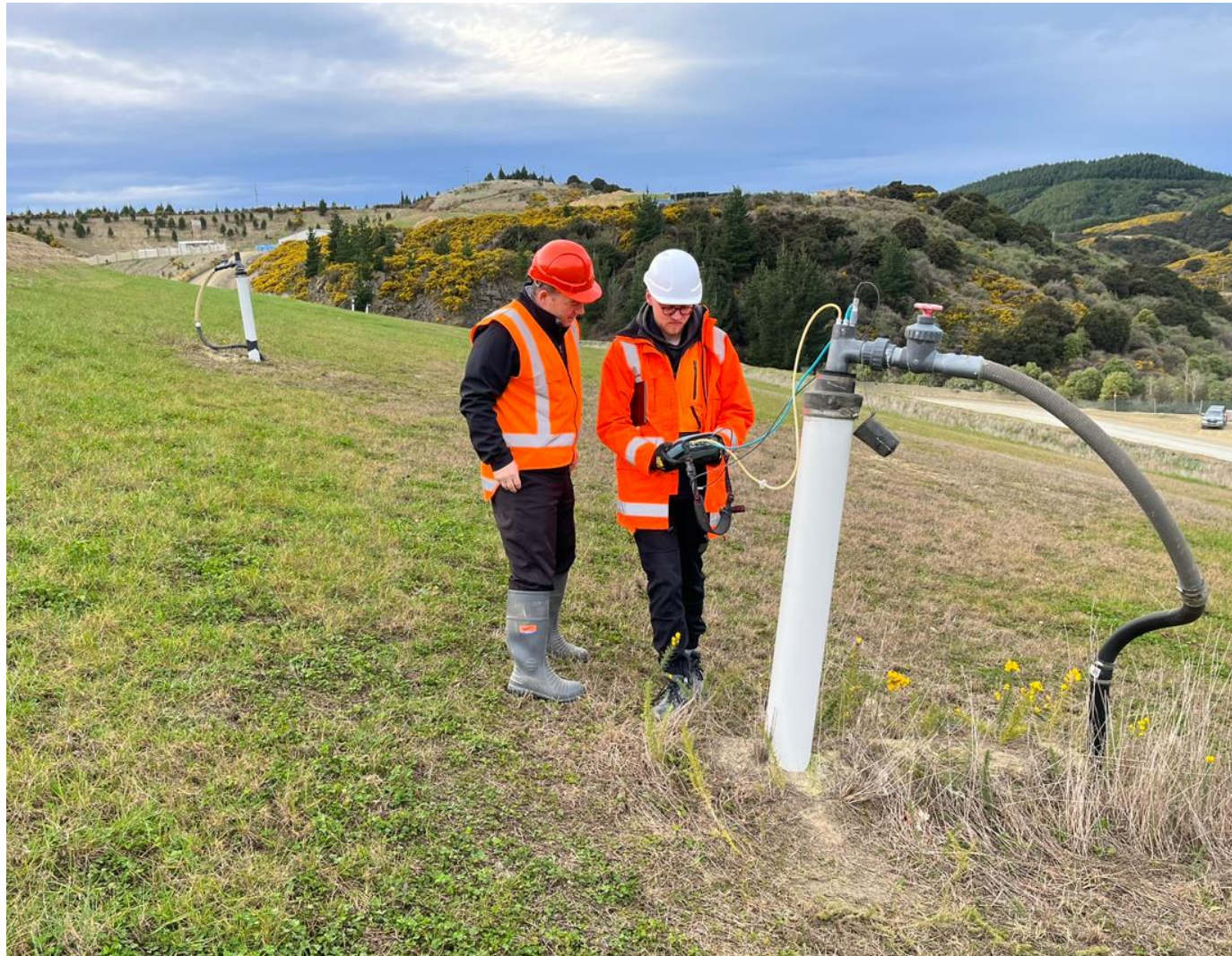
LFG monitoring at a well head
