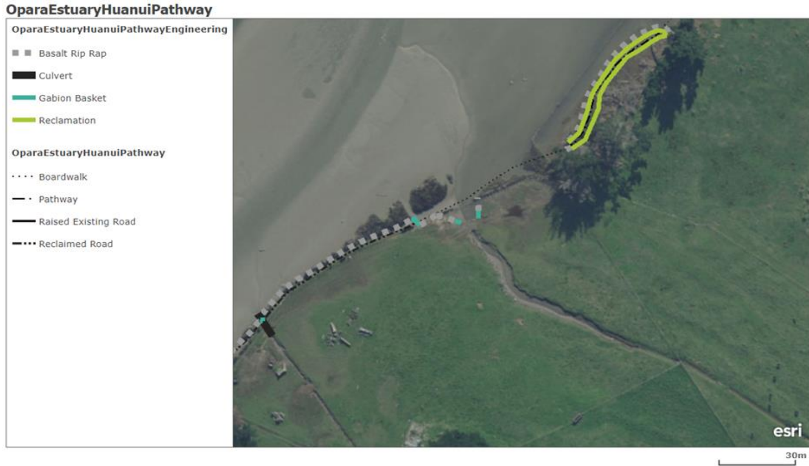
Figure 19: Opara Estuary Huanui Pathway close-up highlighting the locations of basalt rip rap, culverts, gabion basket, reclamation, boardwalk, pathway, raised existing and reclaimed paper road.
