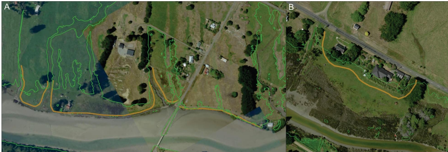
Figure 20: Proposal of inundation bunds to protect low lying assets and productive farmland. Localised protection provides by inundation bunds constructed from excavated sediment from drainage network. Inundation bunds depicted as orange lines extend from lower land areas to meet 1.5 m contour line, depicted as green lines. A) Areas at low lying levels proximal to Chorlton Road Bridge. B) Low lying areas of St John the Evangelist Church and the Vicarage.
