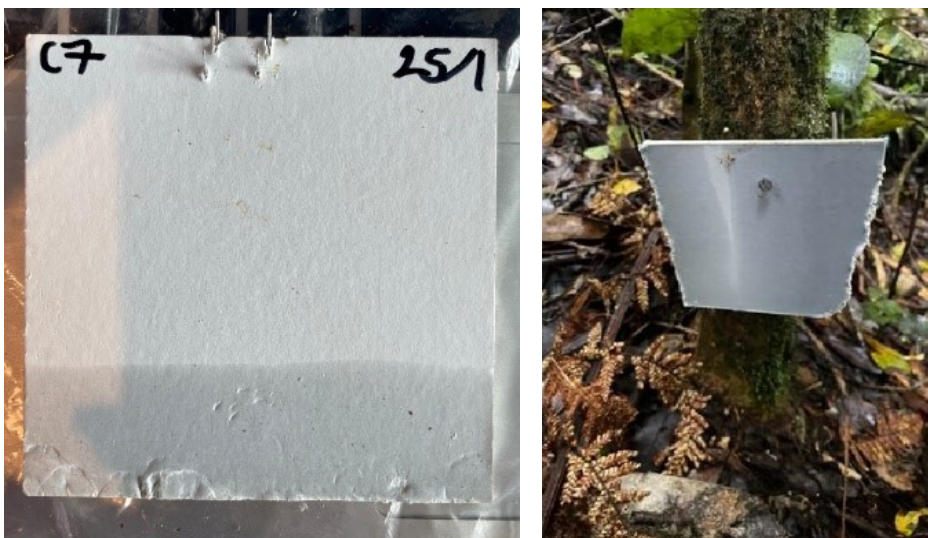
Picture 2: Biodegradable wood- based card alternative prototype.
