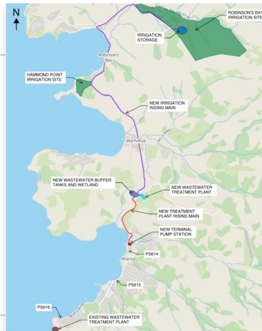
Figure 1-1: Overview Schematic of Akaroa Wastewater Scheme Upgrade
