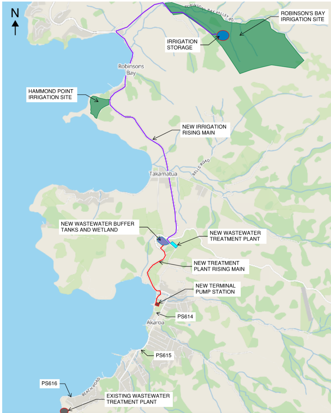
Figure 1-1: Overview Schematic of Akaroa Wastewater Scheme Upgrade
