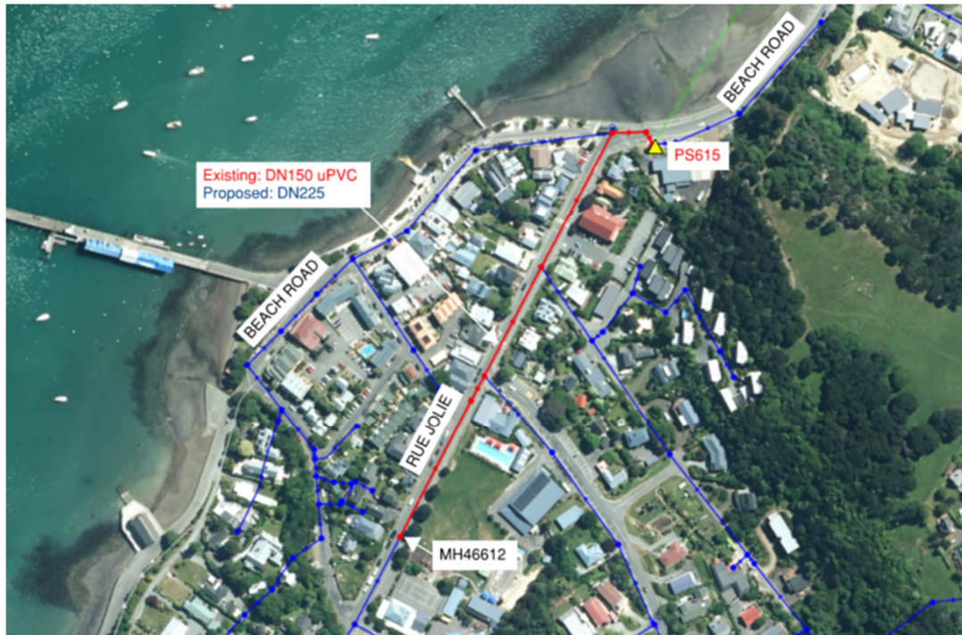
Figure 4-2: DN225 Pipe Upgrades (in red) on Rue Jolie.
