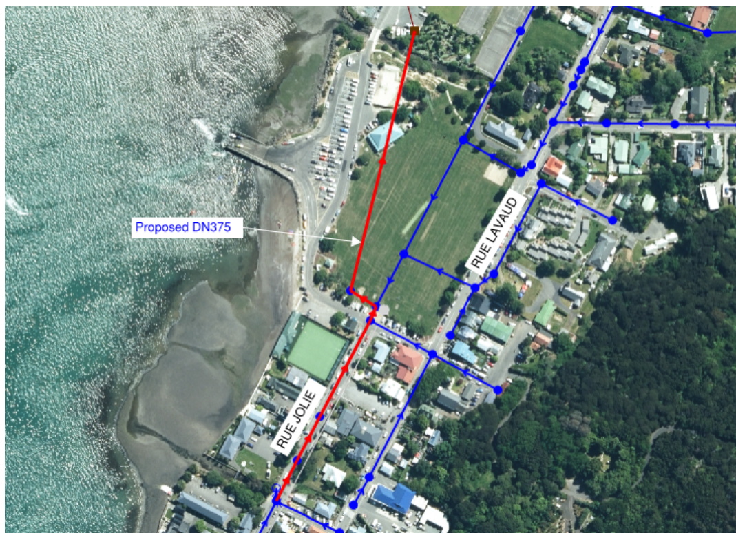
Figure 4-3: DN375 Proposed Pipe (in red) Connecting into the TPS.
