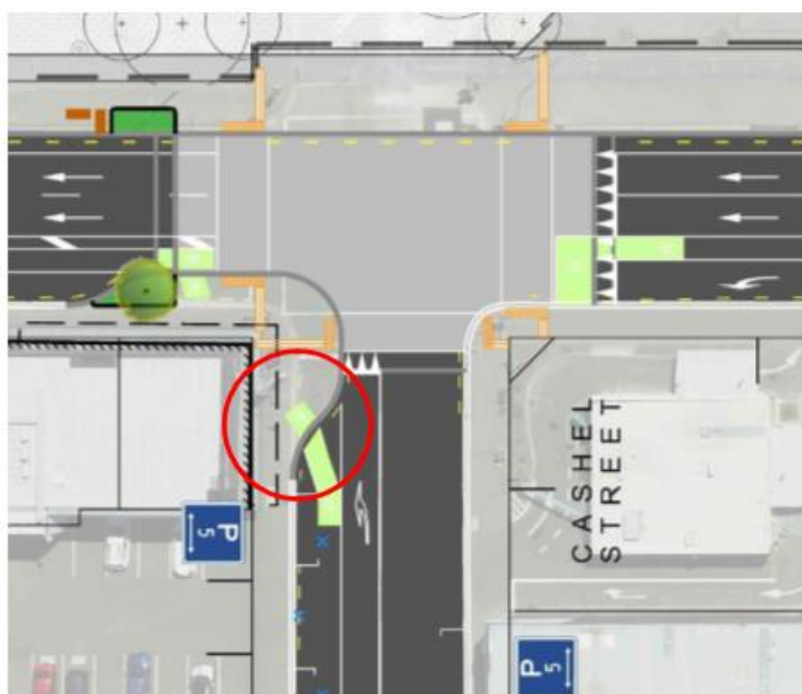
Figure 6-3: The Cashel Street cycle ramp-off facility terminates exactly in line with the existing power pole
