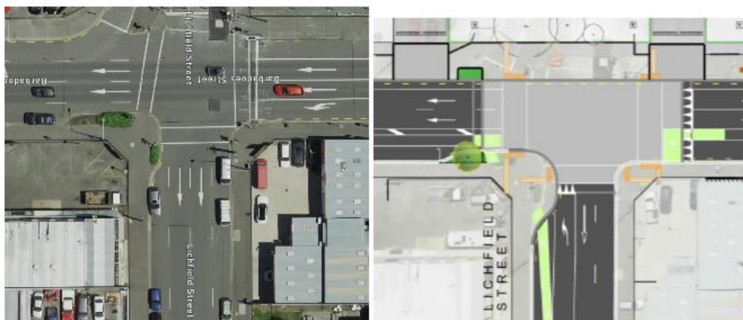
Figure 2-2: The current (left) and proposed (right) layouts of the Barbadoes/Lichfield intersection
