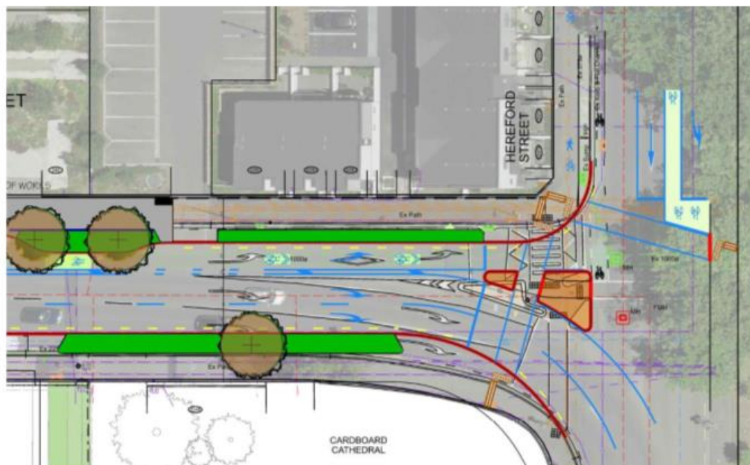
Figure 4-4: Proposed intersection configuration for the Madras / Hereford intersection
