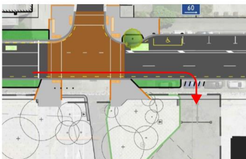
Figure 4-5: The relatively sharp turn required to access the service entrance on Madras Street, and the short holding distance to the barrier arm.
