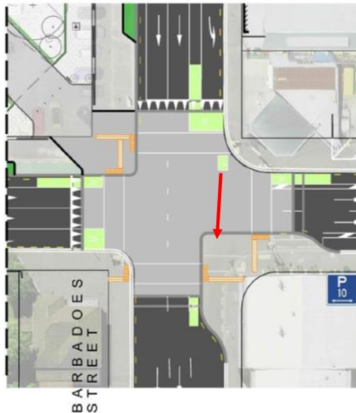
Figure 5-4: Exposed hook turn box in the Tuam/Barbadoes Intersection
