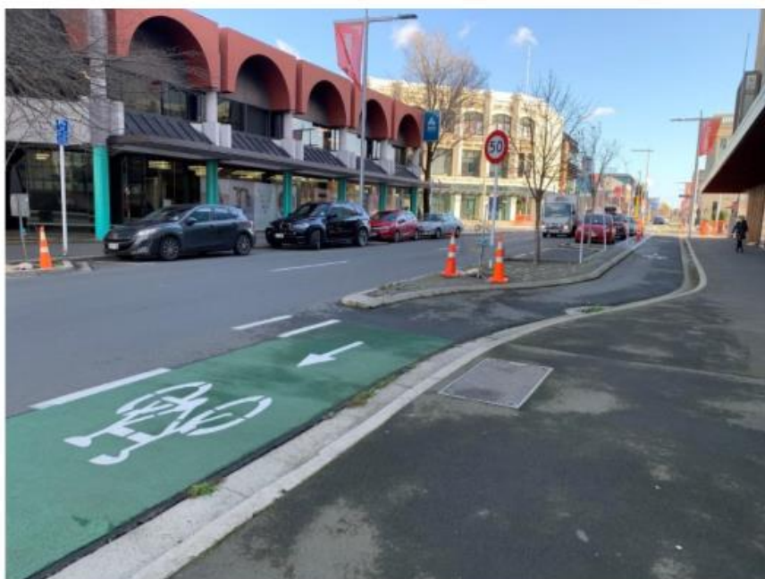
Figure 5-2: The Tuam Street cycleway transitions from separated to on-street at the Nurseryman Lane accessway
