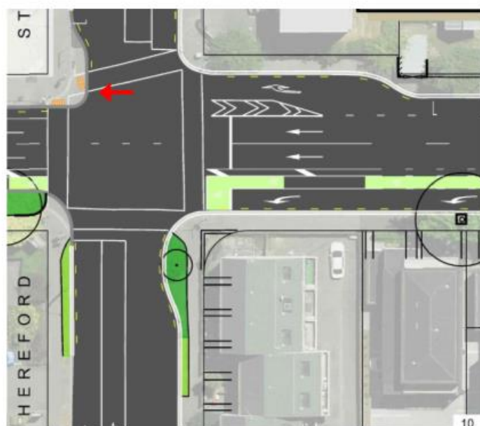
Figure 6-4: Short stack right turn bay and skew crossing at the Hereford Street intersection, the red arrow showing where waiting pedestrians are exposed
