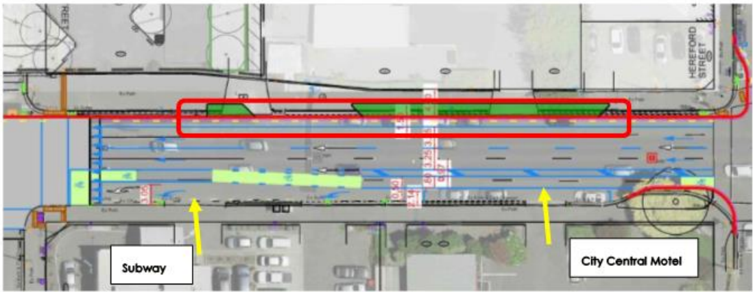
Figure 6-6: The red box shows an area of footpath particularly constrained by a landscaped bed south of the Hereford Street intersection. The yellow arrows show the high volume accesses
