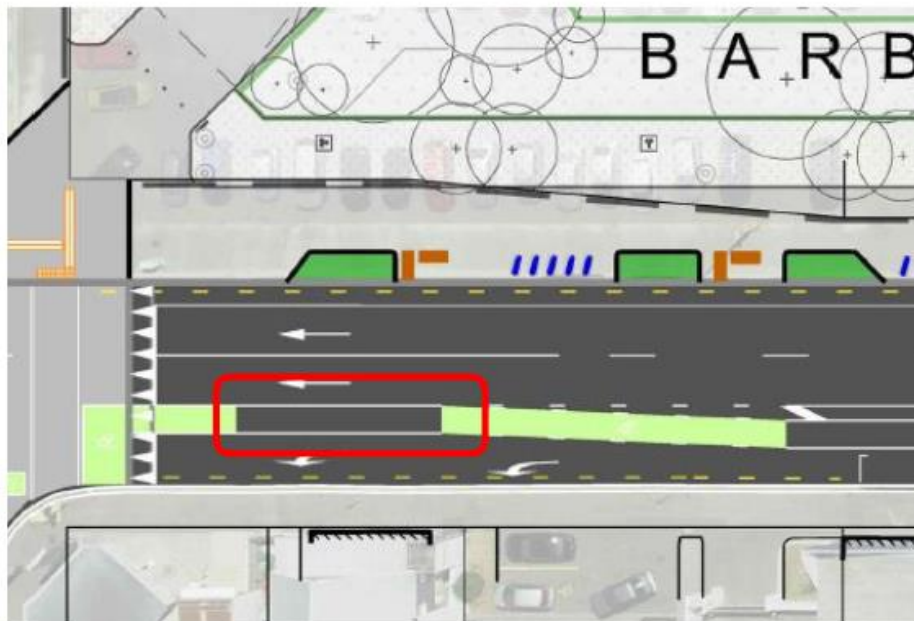
Figure 6-2: Example of incomplete cycle lane green treatment at Tuam/ Barbadoes intersection
