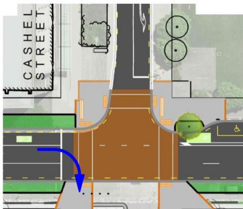
Figure 2-3: And example of poor cycle integration at the intersection of Madras and Cashel Streets; there is no facility for cyclists to move from the on-road cycleway onto the crossing points and into the arena
