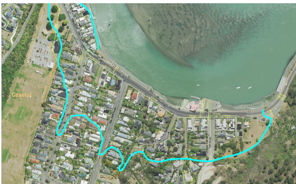
Figure 14: The estimated extent of rainfall-sourced land flooding experienced once in 20 to 50 years. Based on the extent of flooding in March 2014. The majority of house floors are higher than the indicated flood level.
