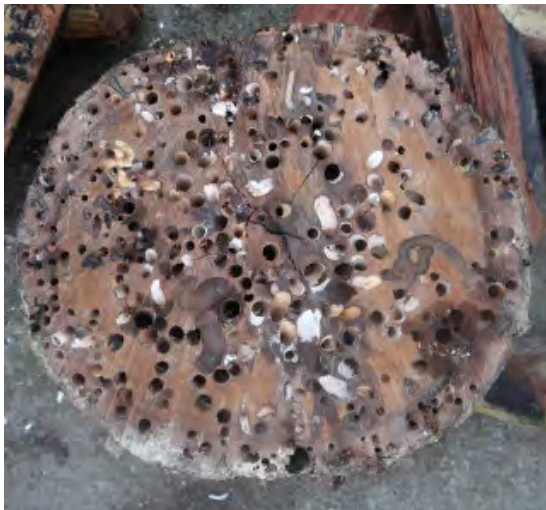
Figure 11: Marine borer damage to hardwood pile
