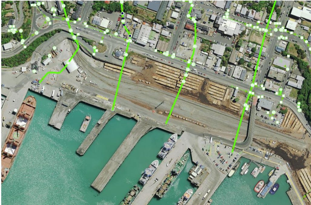
Figure 2 CCC Stormwater pipes in LPC's landholder with hard stand and log yards above. Image from CCC's GIS ( https://gis.ccc.govt.nz/portal/apps/webappviewer/index.html?id=c4ff85ba75724391ae89fbf5f773e00d ) on 14/01/2022.
