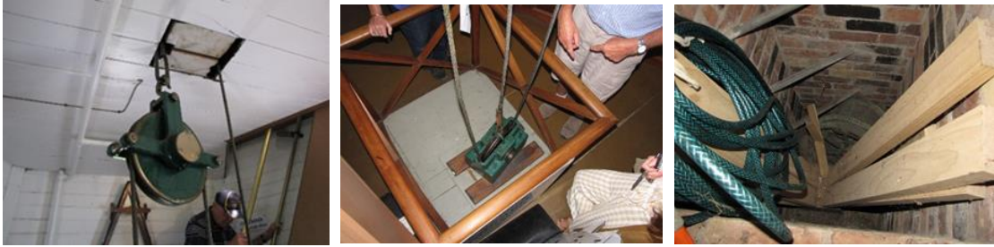
Winding mechanism including the weight pit. These are to be glazed and lit for public viewing.
