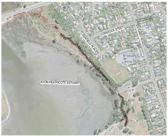
Figure 1 Set Back Bund Layout (black lines show works extent and dark red lines show construction corridor extent)
