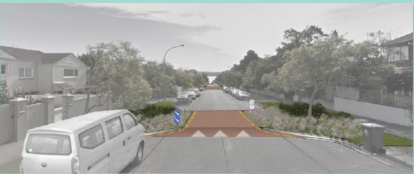
Mid block raised platform with road narrowing
