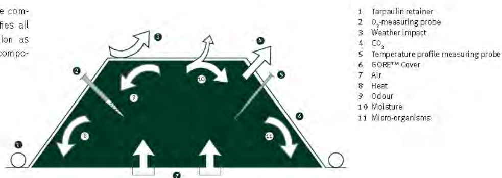
Figure 8 - Gore (R) Cover Membrane Function
