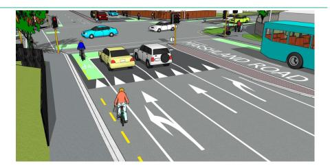
Speed surveys have also recently been completed (December 2023) at the new platforms at the intersection of Briggs/Marshland/Lake Terrace. The survey showed that the average free flow speed recorded on the Marshland Road approaches was 31.2km/h and 28.5km/h on Briggs Road.
