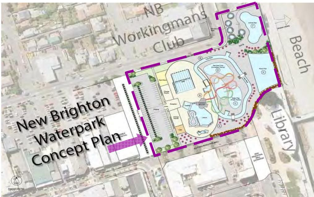
**Waterpark concept**— image from website. This was the initial concept to ascertain what might fit on this area of land. The concept is being further developed. The initial concept incorporates slides, a wave pool, lazy river, 25m lap pool and other play pools. The proposal acknowledges the new road proposed in the Draft Master Plan. Parking is shown alongside the new road. Pools and slides extend across Marine Parade and foreshore area.
